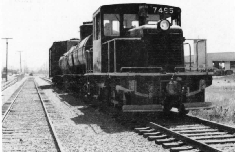
PSRMA's 45 ton side rod diesel clanks by with a three car "drag". Jim Lundquist is at the throttle.
