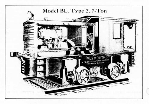
No photos are known to the staff of the REPORT of the narrow gauge railway of the Fenton Material Co. This photo, copied from a Plymouth catalog, shows a Plymouth Model BL seven-ton dinky similar to the two owned by Fenton. The locomotive pictured, however, is standard gauge; the Fenton machines would have the wheels inside the frame.
